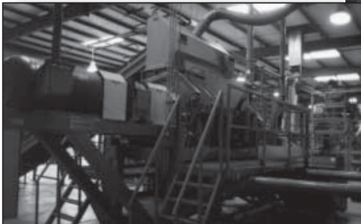
(Below) A Granutech Grizzly takes primary chips down to 1/2-inch minus and liberates steel prior to granulation
