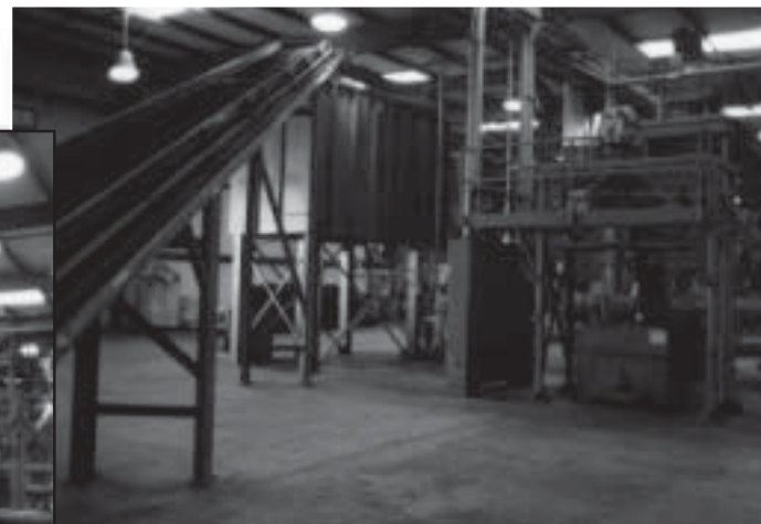
(Above) Material leaves the Grizzly and is routed to a hopper prior to processing.
